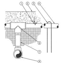
8. LATERAL HEADER PIPE SXT TEE OR ELL, SIZE AND DEPTH PER LEGEND. USE MANUFACTURER TOOL TO INSERT EMITTER DIRECTLY INTO DISTRIBUTION FEEDER TUBE. ALL THREADED CONNECTIONS TO HAVE TEFLON TAPE OR PASTE.
